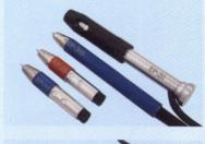
The ITM-525 consists of a basic unit offering a variety of probe sizes. Eddy current probes for through-holes are detachable, consisting of a probe holder with replaceable EP-25 and EP-30 plug-in cartridges. The EP-20 probe is not detachable. Probe tips\* are inserted into through-holes to take readings. Due to the special construction of probe tips, cracks in the copper can be detected. Shortened probes EP-25S and EP-30S are available.
