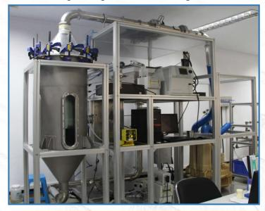
Flow resistance Test Rig
